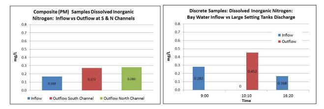
Figure 10. Composite DIN results both channels (left) and discrete DIN: Large Setting Tanks (right).
