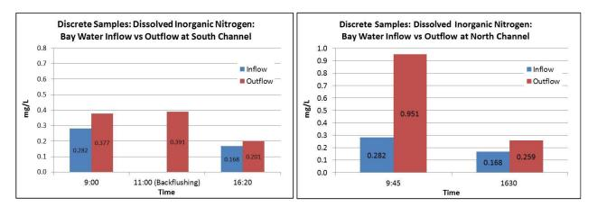
Figure 9. Discrete DIN South Channel results (left) and North Channel (right).
