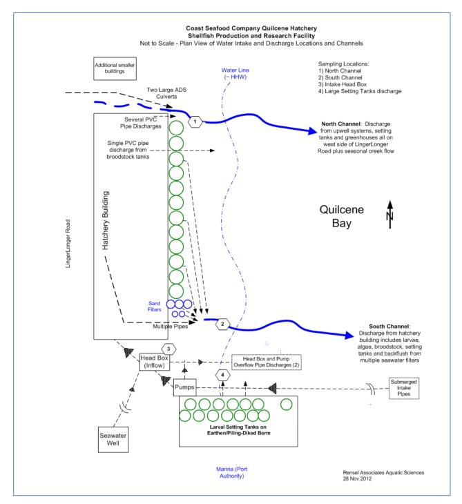
**Figure 4.** Schematic layout of Coast Seafoods Company facilities near the shoreline of Quilcene Bay. Not to scale.
